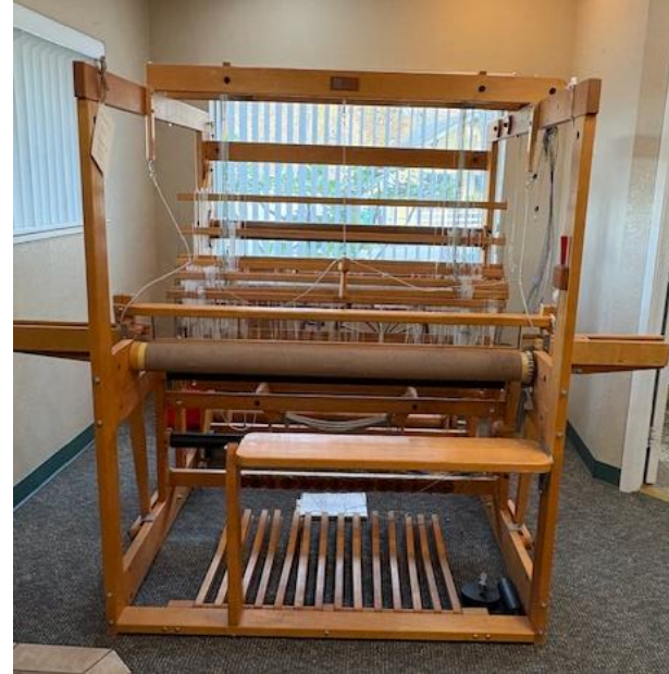
Gloria is a 12-shaft manual AVL loom with shuttle race. Donated by Gloria Novak, this loom will enable weavers to take on almost any complex weave structure or produce yards of cloth.
