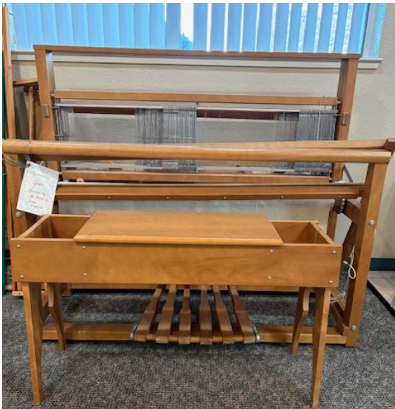
Jean is a 4-shaft, jack loom. This is another great floor loom that will enable weavers to develop skills on a wide array of projects.
